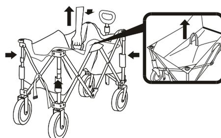
Take out the plates, and pull upwards on the handle in the middle of the bottom to fold the cart.
