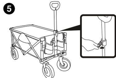
5. Release the red locking mechanism, pull out the handle to extend to maximum length, then push down on the lock to secure for use.
