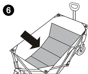
6. Put the plates on the bottom of cart.
